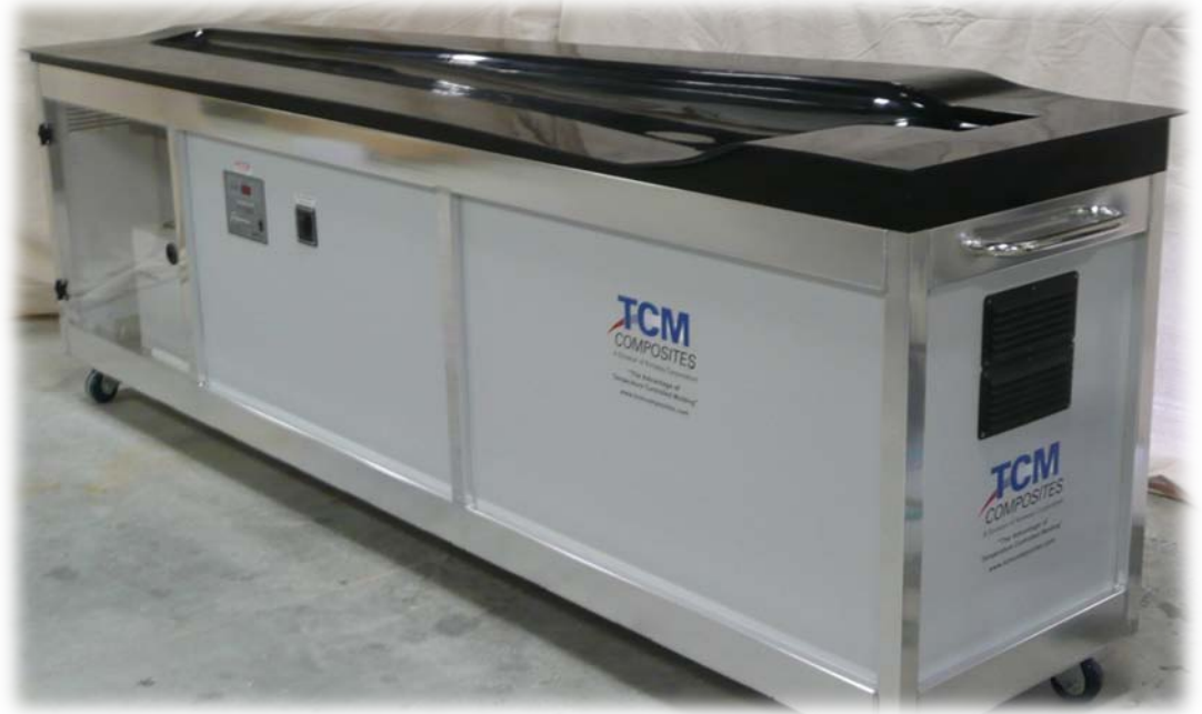
Small Scale Prototype Windblade Mold
