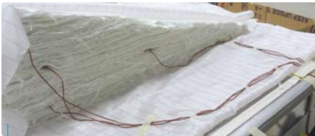
In one of many experiments during trials of the thick-part curing technology, the development team infused a wedge-shaped laminate stack. This photo shows the placement of thermocouples within the stack to monitor exotherm in real time during the cure cycle. ■
