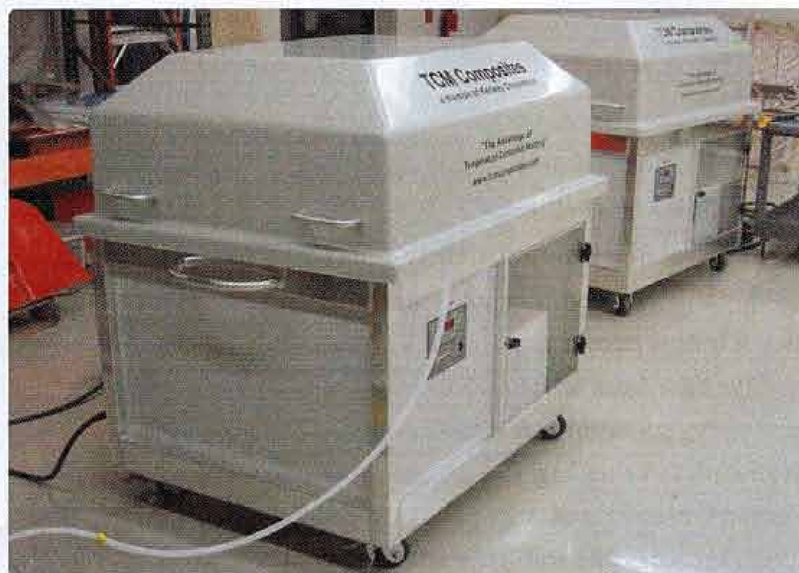
6 During cure, the stacks are enclosed in these temperature-controlled closed molds (the chart on p. 37 tracks exotherm during a typical cure cycle). Developed by ACSM and Kenway's new TCM Composites division, these units will be used by ACSM as the company trains customers to use the new BlocBuilder technology. ■
