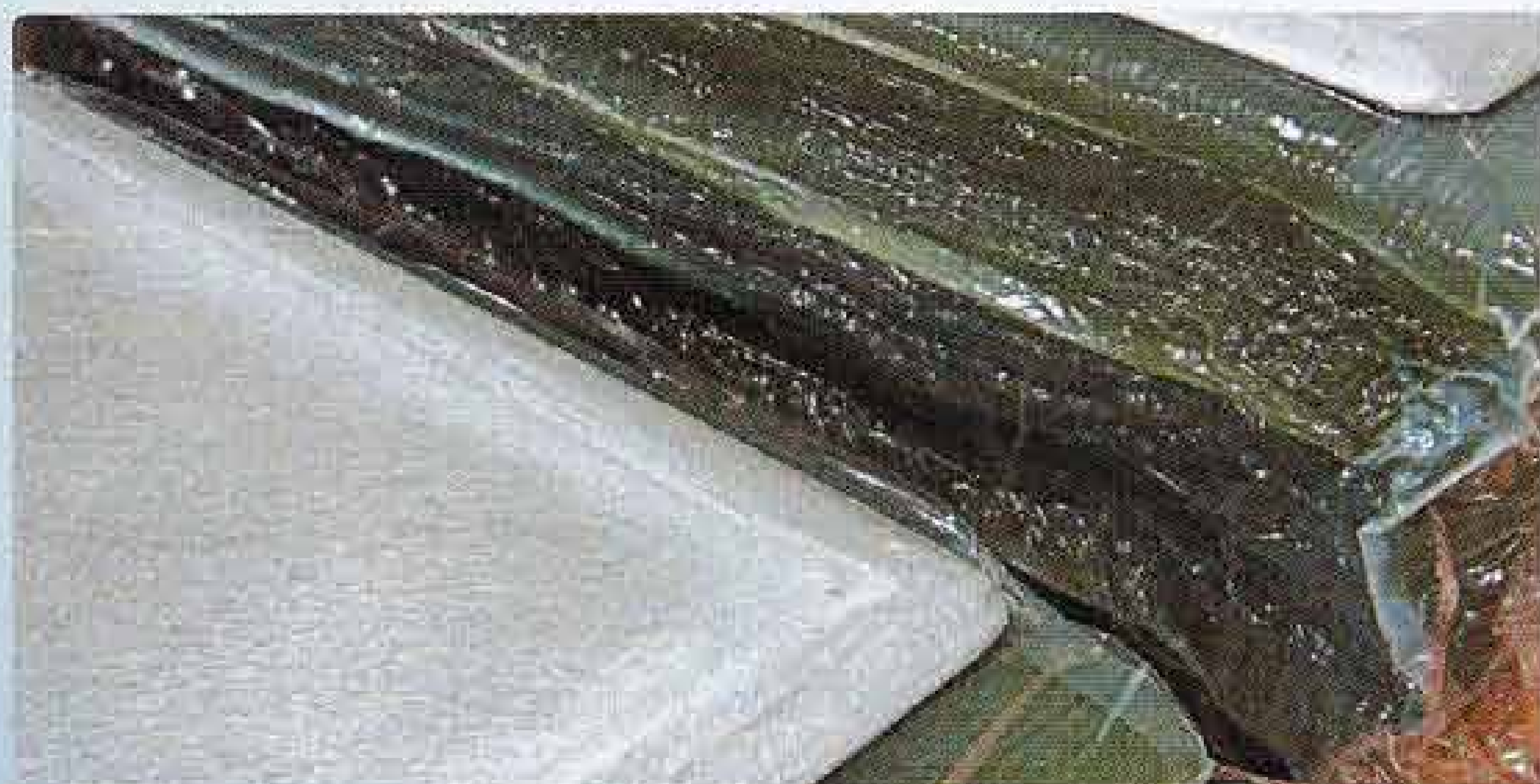
4 This close-up shows that wetout is complete. The laminate stack is found to have no dry spots or air pockets. ■
