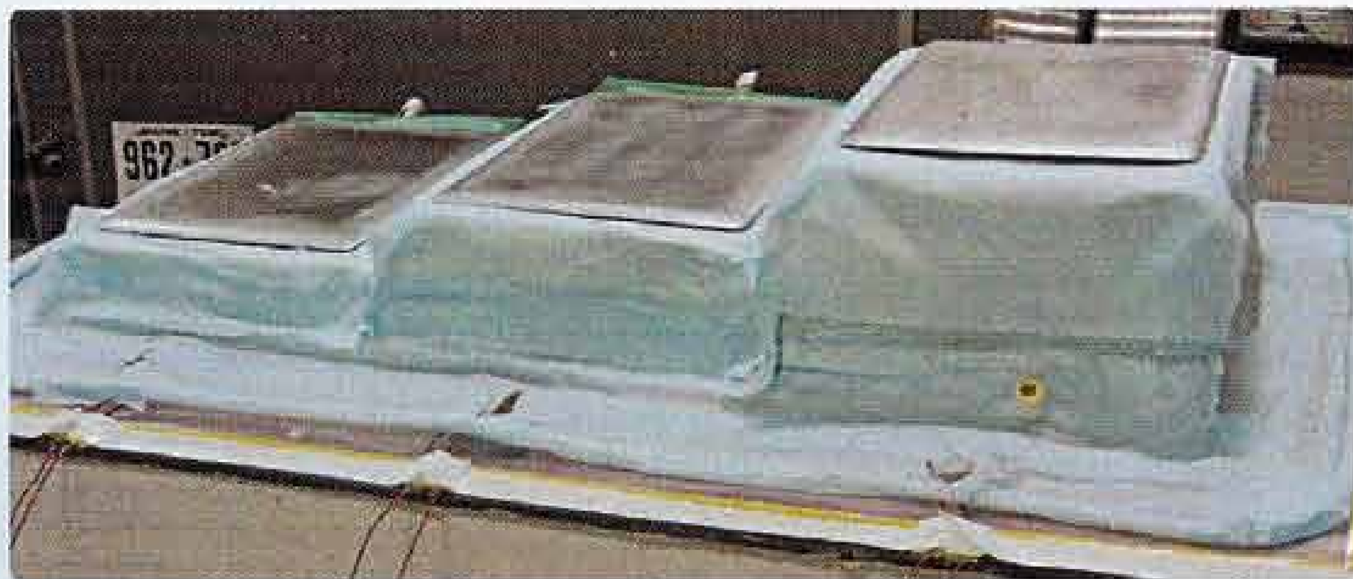
2 Three laminate stacks — 2, 4 and 6 inches in thickness (51 mm, 102 mm and 152 mm) — topped by steel caul plates are readied for simultaneous vacuum infusion under a single vacuum bag. ■
