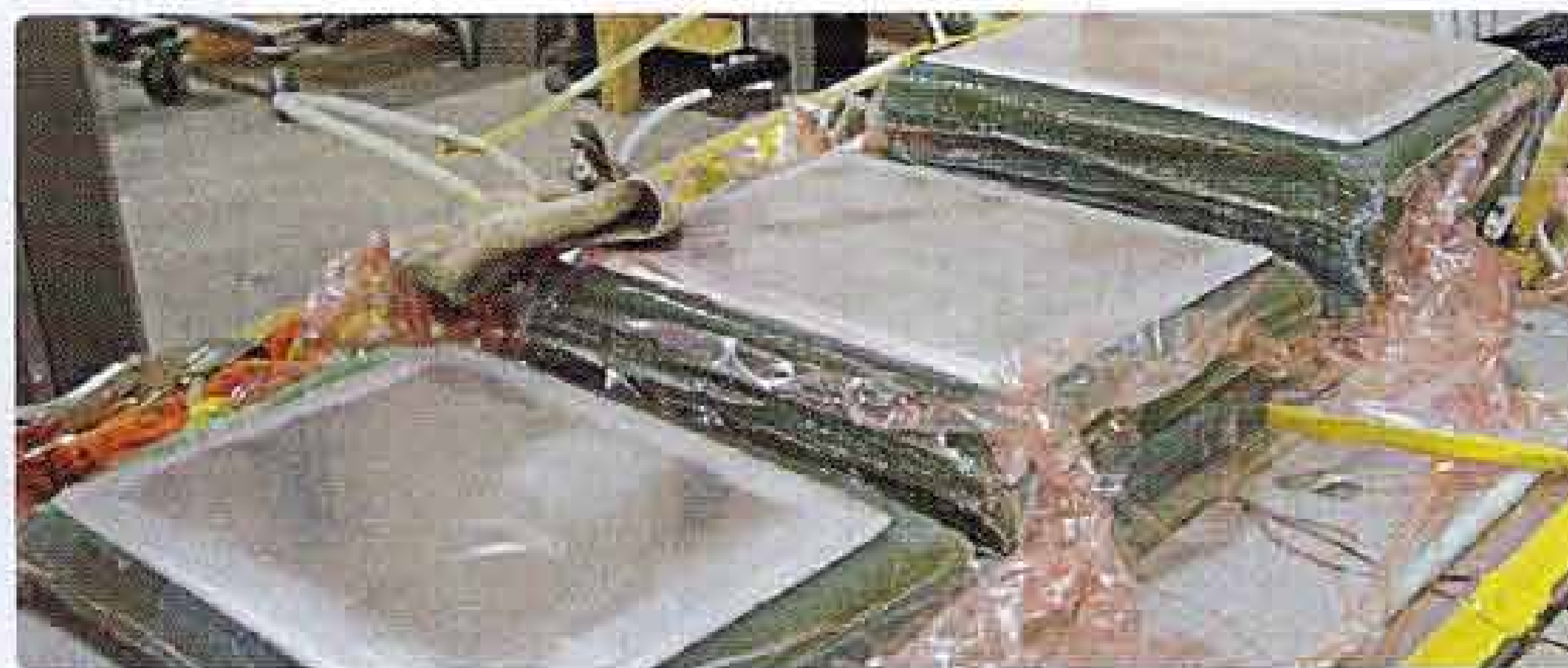
5 The completely infused stacks are ready for cure initiation, accomplished by heating the mold table. Cure will be triggered as the temperature reaches a predetermined level. ■
