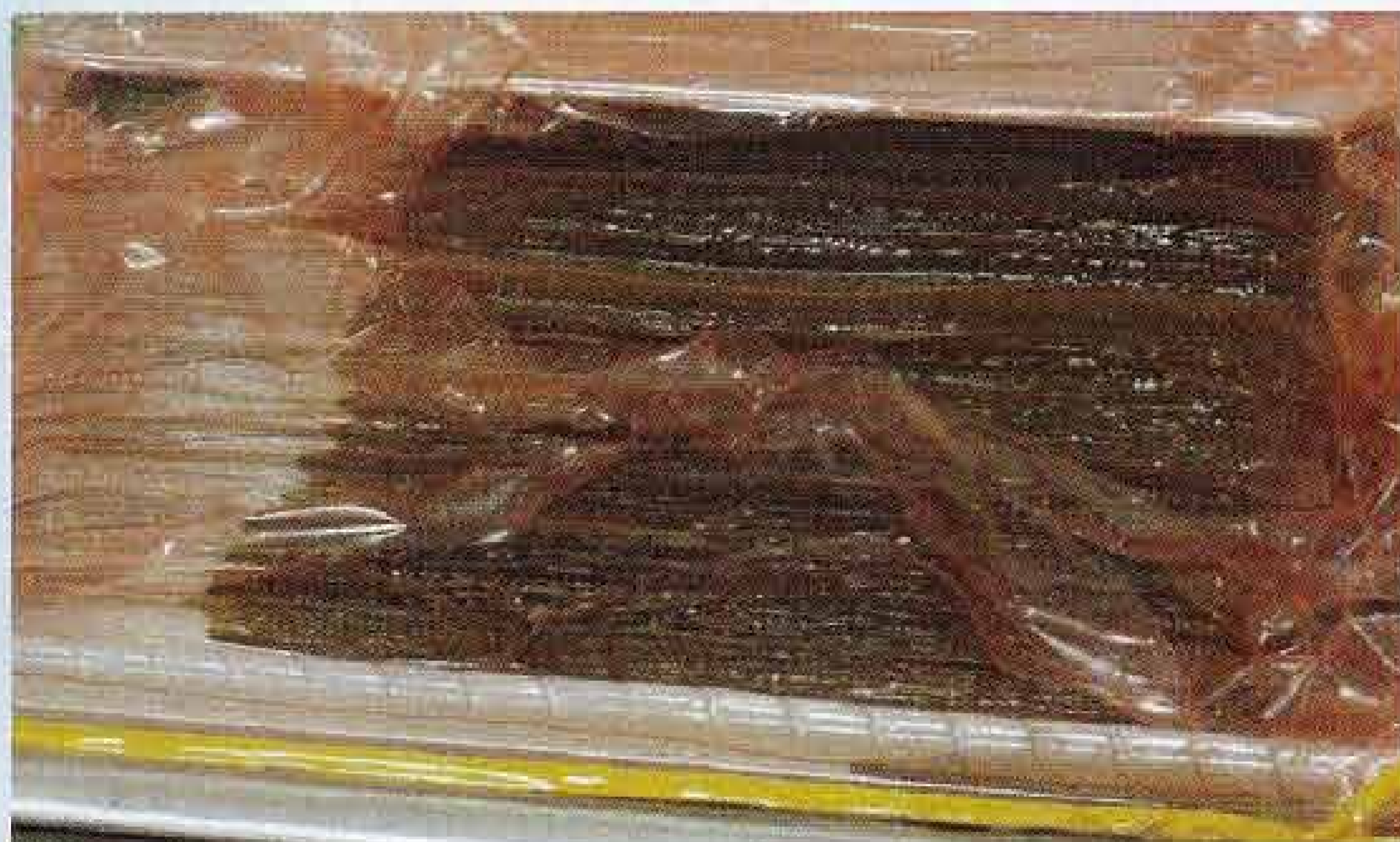
3 Infusion begins. This close-up shows the BlocBuilder-modified vinyl ester resin front moving through the thick fiberglass laminate stack. ■
