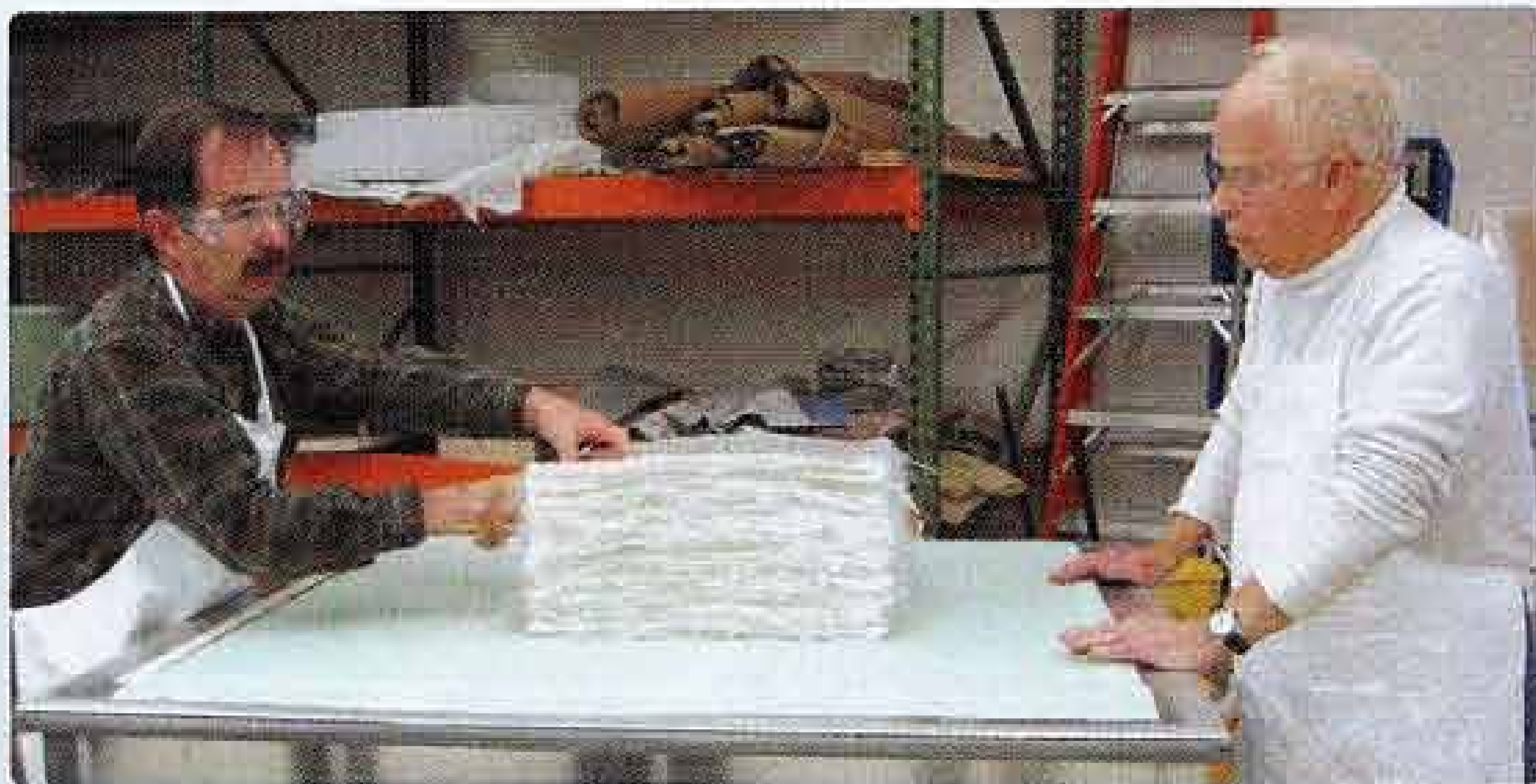
1 A 6-inch/152-mm laminate stack, consisting of 90 fiberglass plies, is layed up on a temperature controlled flat-table mold. ■
